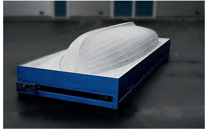
Fig. 4. An approx. 2500 kg, high-quality thermoforming boat-mold that can be molded perfectly, even at the edges
